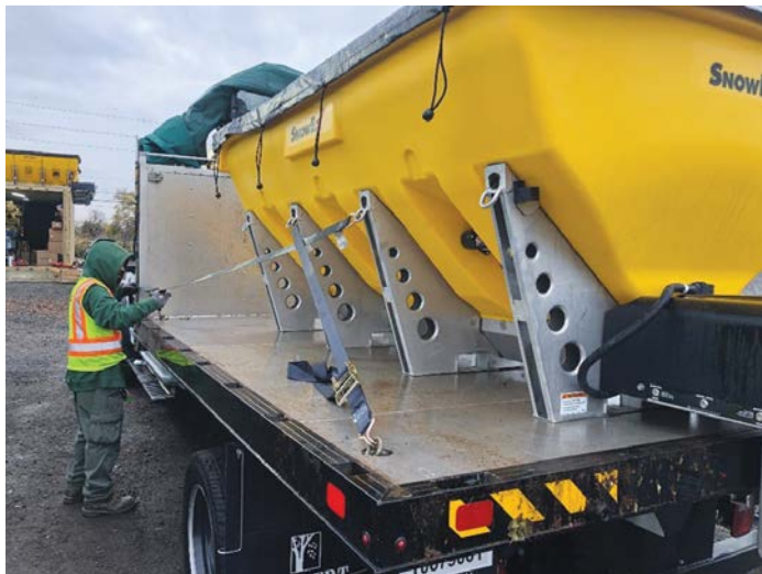
Teams mounting salt spreaders and plows to ensure they are working and properly secured to the trucks.
