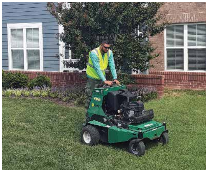
A new type of stand-on aerator that is faster and creates less fatigue for the operator.
